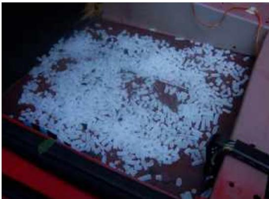
Continue usage of rubber mallet until most bits are loose. Clear out the chunks and then put the dry ice back on the last few bits. Grab another coffee, if so inclined, and wander into the shed to find a large flat bladed screwdriver. With screwdriver in hand, return to the car, remove the pellets and pry up the last remaining pieces of the semi-frozen tar.
